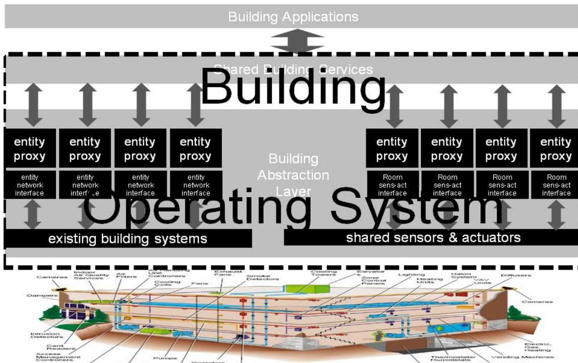
Sensors and actuators are supposed to be shared between all building applications and made available as a pool when they are individually identifiable and addressable (right-hand side of the diagram). Black box legacy systems that do not give access to their individual sensors and actuators will be dealt with through their own interfaces (left-hand side of the diagram).
